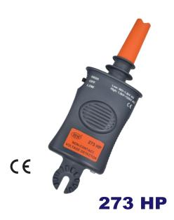
The 273 HP is a Non-contact voltage detector. It has two ranges for selection. The 273 HP consists of an internal pickup sensor, a function selection switch, a visual and a sound annunciator. With the 273 HP, physical contact with electrical conductors is not necessary when testing for live lines.
